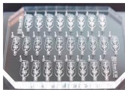
Fig. 2. Standard Drop-sequencing chip containing 26 individual Droplet Generation Devices.
